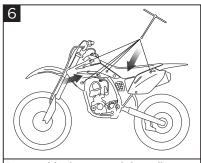
Reassemble the seat and the radiator scoop.
