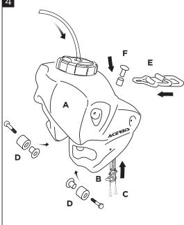
(1) Install the acerbis petcock. (2) Place the acerbis tank. (3) Replace the grommets with sleeve. (4) Instal the seat screw and elastic attach.
